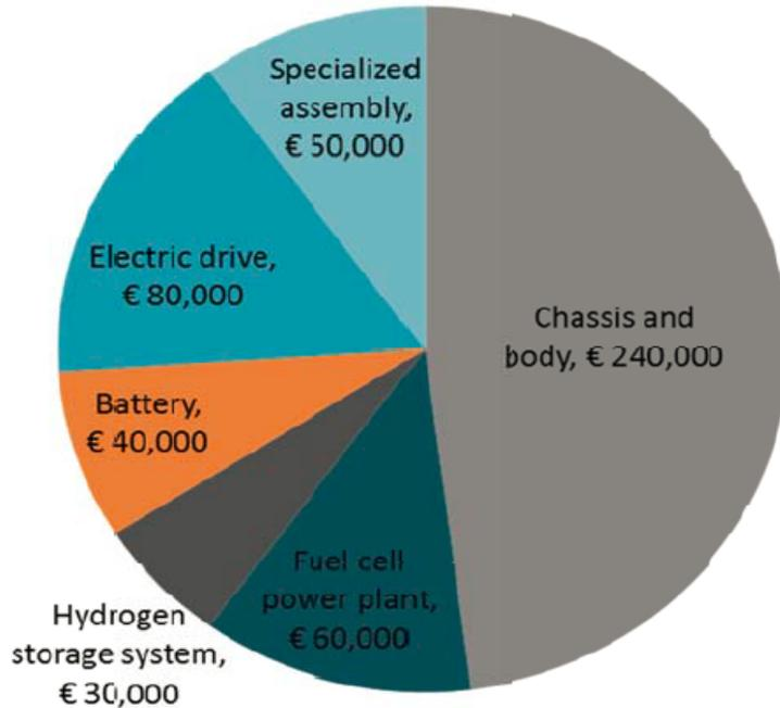
Figure 6: Fuel cell electric bus component cost estimate with 60kW fuel cell power module (2020)
